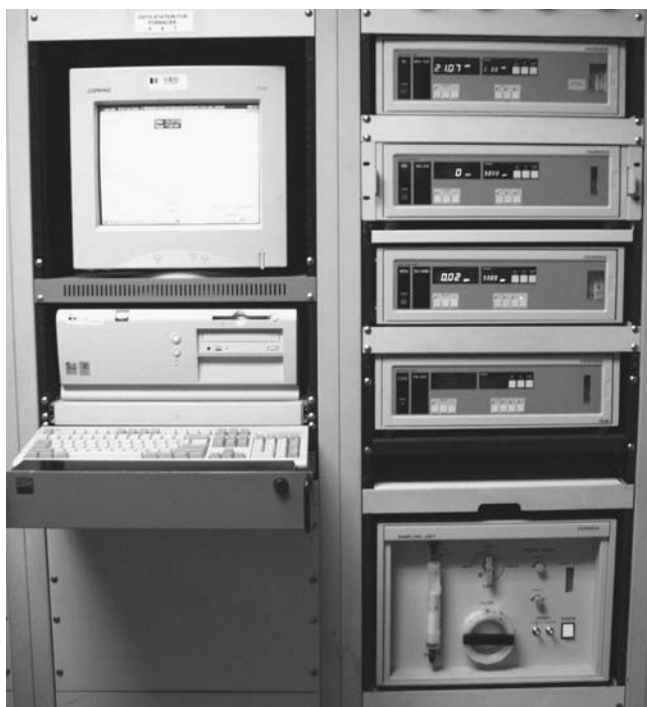
FIGURE 9.12 Gas sample analysis system.
