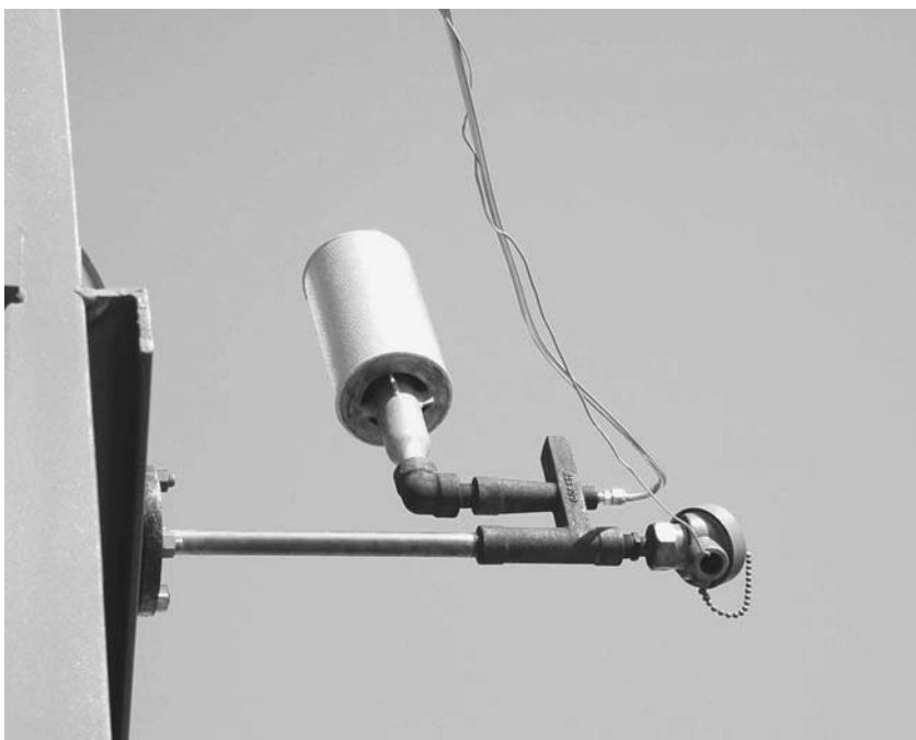
FIGURE 9.8 Suction pyrometer with noise muffler.
