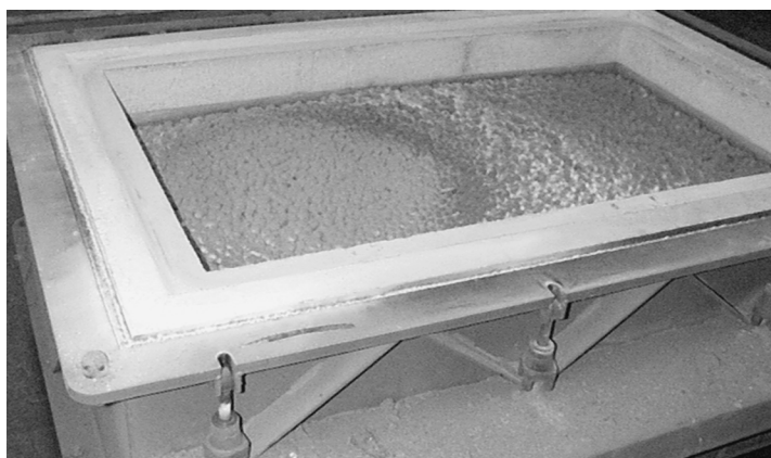
FIGURE 12.13 An aluminum melter's cassette regenerator being removed by forklift truck.
