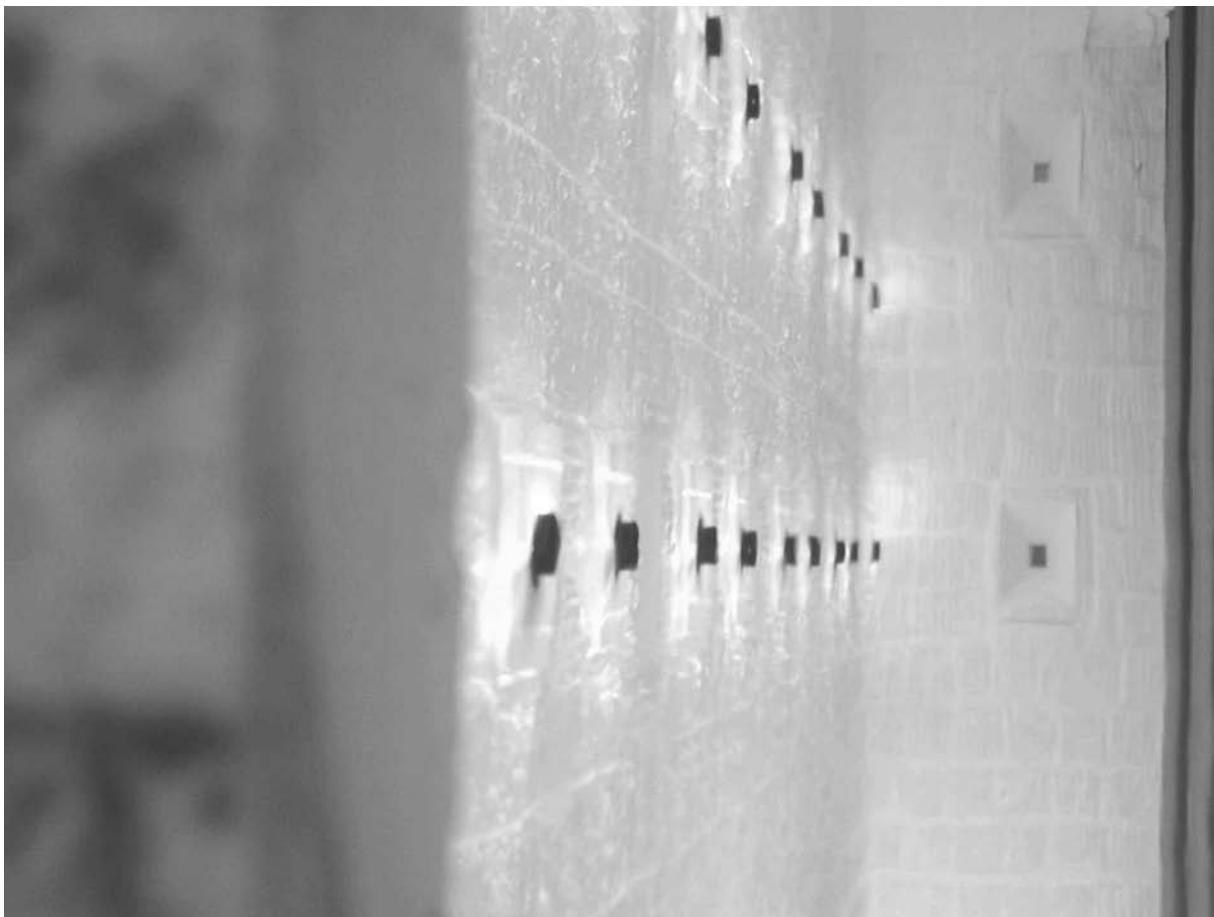
FIGURE 15.1 Radiant wall burners (natural draft) firing in an ethylene-cracking furnace. (Courtesy of John Zink Co., LLC.)
