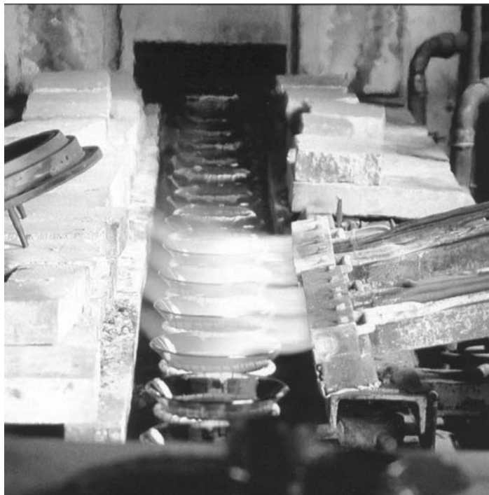
FIGURE 21.27 Glass flame polishing production line.
